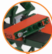
Inclined Conveyor with Overhead Magnetic Cross- Belt for Ferrous Removal
