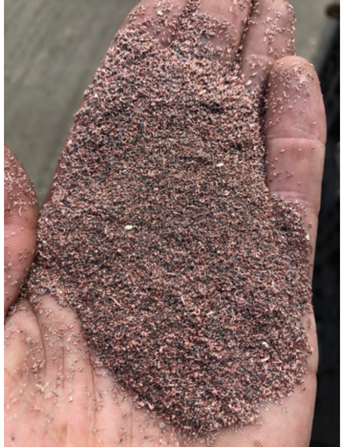
The end product from mixed low yield ICW after running through SWEED Turbo Mill.
