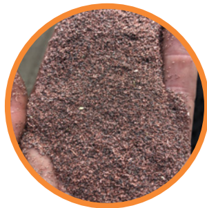
The end product from mixed low yield ICW after running through SWEED Turbo Mill.
